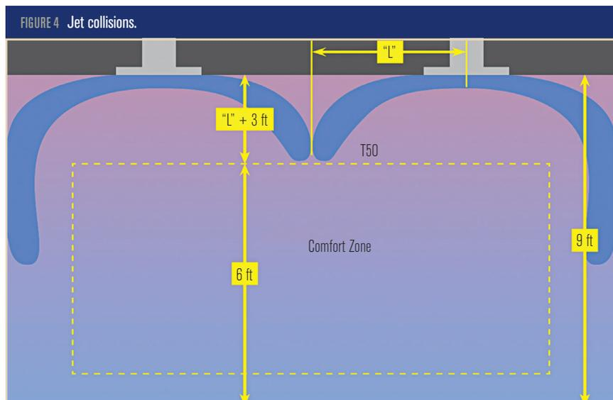
It is reduced the farther away the jet is from the air outlet. If the jet is cooler, and thus denser, than the room air, it will detach from the ceiling when the forward momentum of the supply jet is less than the downwards buoyancy force. If the buoyancy force is great enough, the supply jet may enter the occupied zone with an objectionable temperature or velocity. This effect is predictable and should be considered by the designer.
